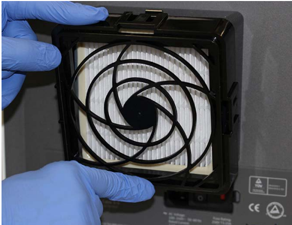
Figure 9-30. Replacing the HE Filter Retainer
