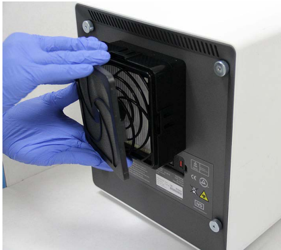
Figure 9-25. Removing the Prefilter Retainer
