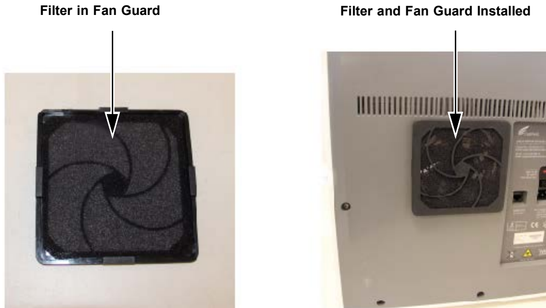
Figure 9-23. Replacing the Filter and Guard
