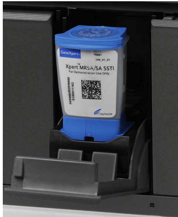
Figure 5-28. GeneXpert Cartridge, Positioned at the Heel of the Module Bay Floor
