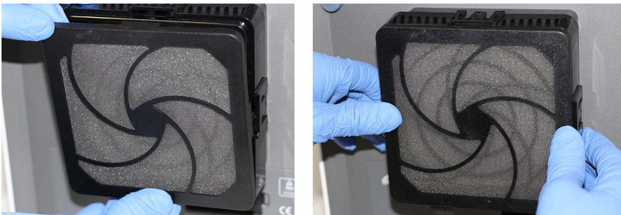
Figure 9-31. Replacing the Prefilter and the Prefilter Retainer
