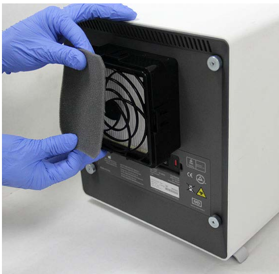
Figure 9-26. Removing the Prefilter
