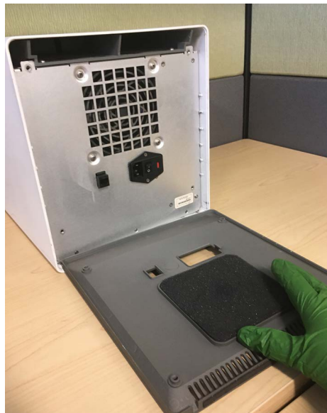
Figure 9-16. Replacing Foam Filter in Older GX-IV
