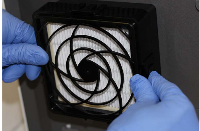
Figure 9-30. Replacing the HE Filter Retainer
