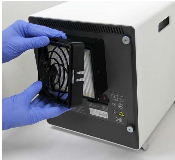
Figure 9-27. Removing the HE Filter Retainer
